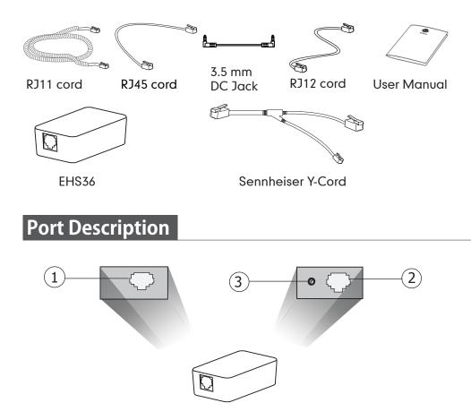
Port (1): Connect with the IP Phone EXT port or Expansion Module port (expansion module connected to the phone) through RJ12 cord.
